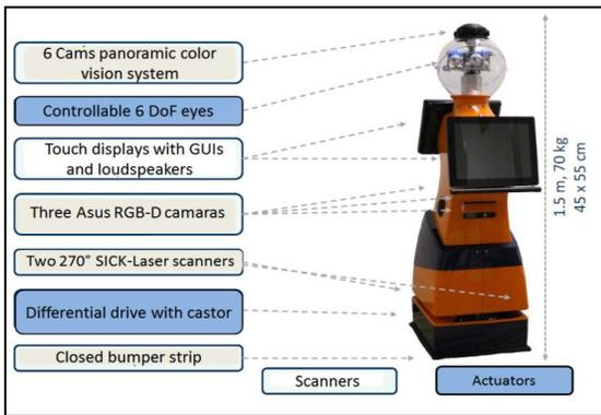
Figure 5. ROREAS demonstrator consisting of the SCITOS platform (MetraLabs, Ilmenau) with its main equipment for environmental perception; navigation and human recognition (Technical University Ilmenau).
